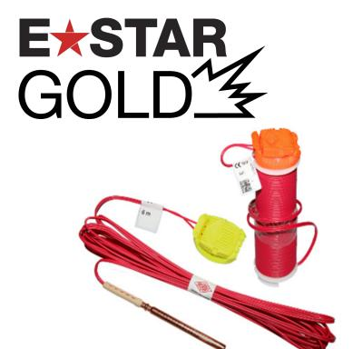
E\*STAR GOLD detonator is characterized by maximum safety, timing accuracy and variability of initiation for most of the blasting applications. Using E\*STAR Logger 2 it is possible to program the detonators to any delay within the range from 1 to 20,000 ms. Using the E\*STAR Blaster it is possible to fire up to 1,600 E\*STAR GOLD detonators per blast. Using E\*STAR Remote Blaster and E\*STAR Remote it is possible to control blast initiation remotely.
